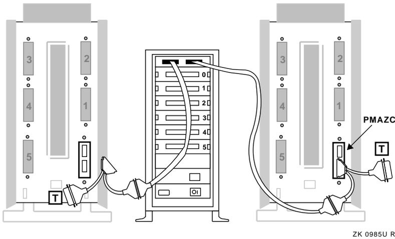
If you have the same hardware as described in Figure 3–9, you can create an alternative hardware configuration by placing one of the systems in the middle of the shared bus and the storage shelf at the end of the bus. In this case, the BA350 storage shelf internal termination is used to terminate the bus, as shown in Figure 3–10.
