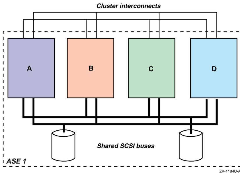
The TruCluster Production Server Software product allows multiple ASEs. Each ASE is numbered individually. All member systems in an ASE must be connected to the same shared SCSI buses. Figure 1–3 shows a four-member Production Server configuration with two ASEs. In this configuration, member systems A and B are in ASE 1 and systems C and D are in ASE 2. The cluster interconnect is the MEMORY CHANNEL and the MEMORY CHANNEL hub, which is not shown.
