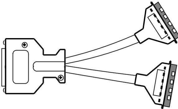
Figure 3-5 shows a BN21W-0B Y cable, which you may attach to a KZTSA or KZPSA SCSI adapter that has had its onboard termination removed. You can use the BN21W-0B Y cable with an HSZ10, HSZ40, or HSZ50 controller. Use a trilink connector with a KZTSA instead of the Y cable.
