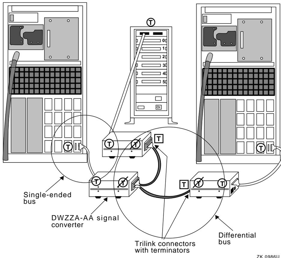
In Figure 3–11, there is a single-ended bus between each single-ended device (KZMSA adapter or BA350 storage shelf) and the single-ended side of a DWZZA-AA signal converter. The single-ended bus is terminated by the internal termination in the device and in the signal converter, as shown in Figure 3–12. If a cable is disconnected from the single-ended device, the
