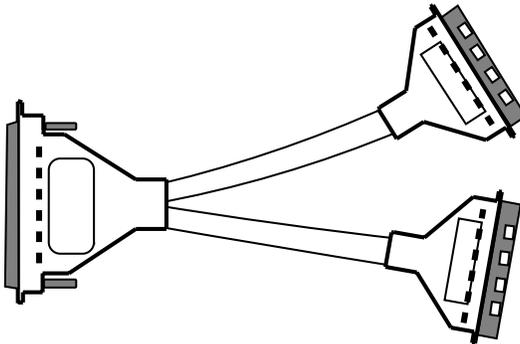
Figure 3-6 shows an HD68 trilink connector (H885), which you may attach to a KZTSA or KZPSA adapter that has its onboard termination removed, an HSZ10, HSZ40, or HSZ50 controller, or the unterminated differential side of a SCSI signal converter.
