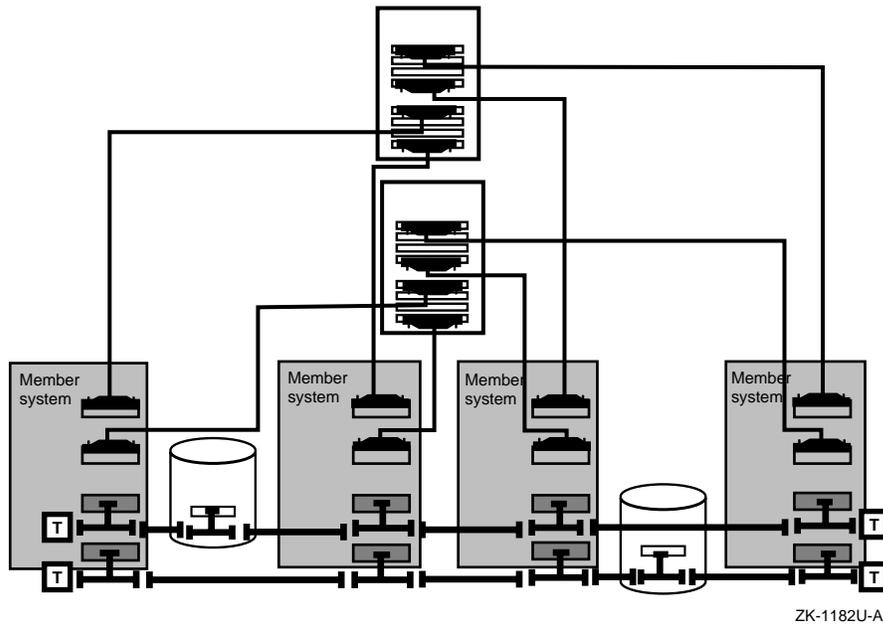
Figure 6–20 shows a Production Server hardware configuration with two ASEs. Each ASE consists of two member systems, each connected to two shared SCSI buses. Each member system also has redundant MEMORY CHANNEL interconnects in a standard hub configuration (including MEMORY CHANNEL hubs). Because this configuration requires four PCI slots, it is not supported on AlphaServer 2000 or 2100 systems.
