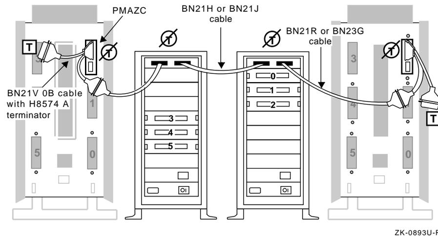
Figure 6-4 shows a configuration consisting of two types of single-ended SCSI controllers and one single-ended storage shelf. This configuration uses a DEC 7000 system, which uses KZMSA XMI-to-SCSI bus adapters. You must use a DWZZA-AA with the KZMSA because the KZMSA does not have removable termination. Therefore, to provide a differential bus for all devices, you must connect SCSI signal converters to each of the single-ended devices.
