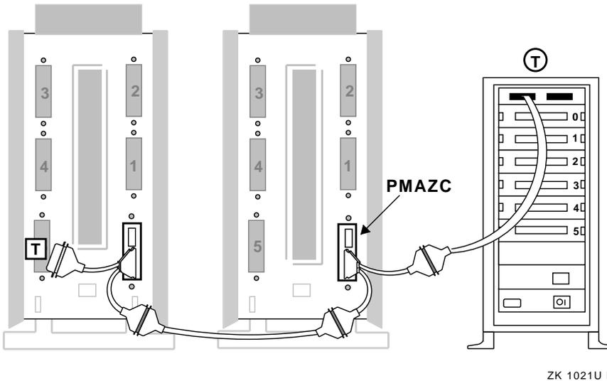
However, if you have the configuration shown in Figure 3–10 and you disconnect the cable from the BA350 storage shelf, the single-ended shared bus is not terminated and ASE operation is impaired. To be able to isolate
